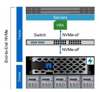
Figure 2) NVMe-oF provides a high-bandwidth, low-latency interconnect between host servers and storage, modernizing your SAN for the next era of computing.
