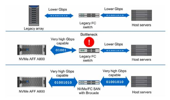
Figure 1) Traditional storage networks can't deliver the bandwidth and the low latency of NVMe SSDs to host servers.
